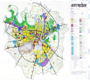
Here ring road around the city has been planned and similar to that a canal adjacent to it is being proposed with a vision to save and monitor supply water that will also provide an alternative transportation means which is economical and eco friendly having a multipurpose solutions.
